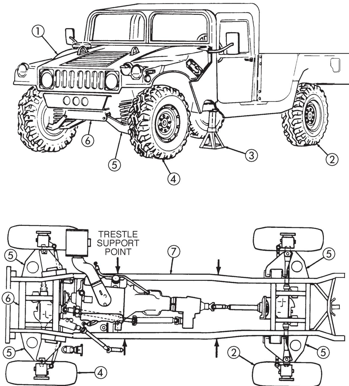
Figure 8-1. Front and Corner Jacking Procedures.
