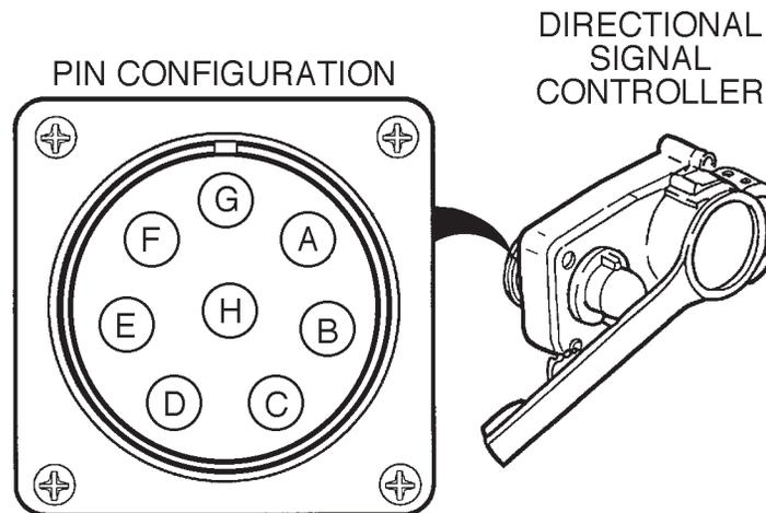
Figure 12-14. Turn Signal Pin Configuration.
