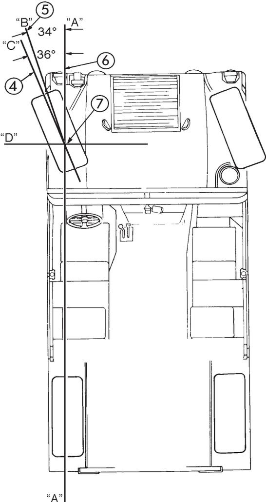
Figure 7-11. Steering Stop Reference line
