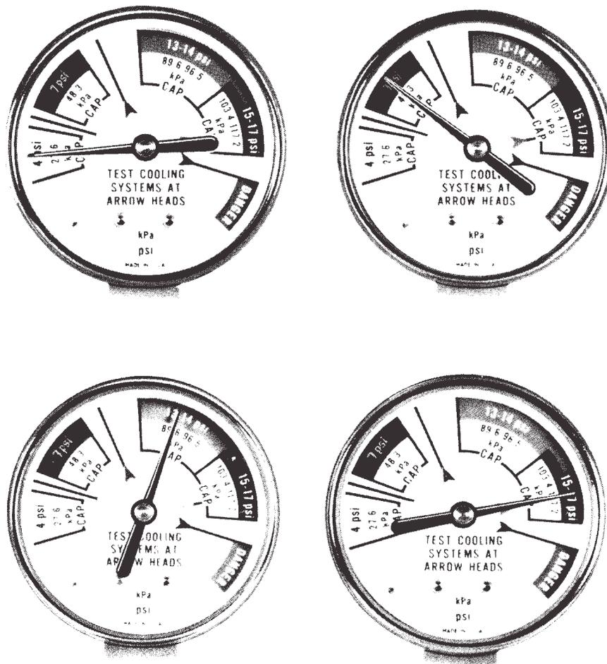
Figure 1-10. Tester Gage Readings.
