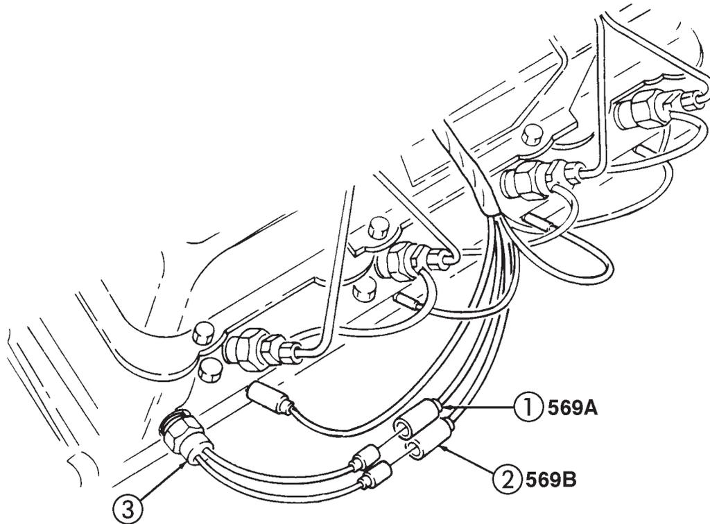
Figure 3-8. Cold Advance Solenoid and Switch Hook-up.
