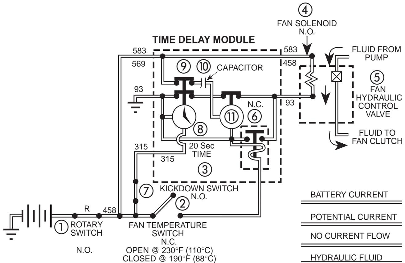
Figure 13-5. Fan Temperature Switch Open
