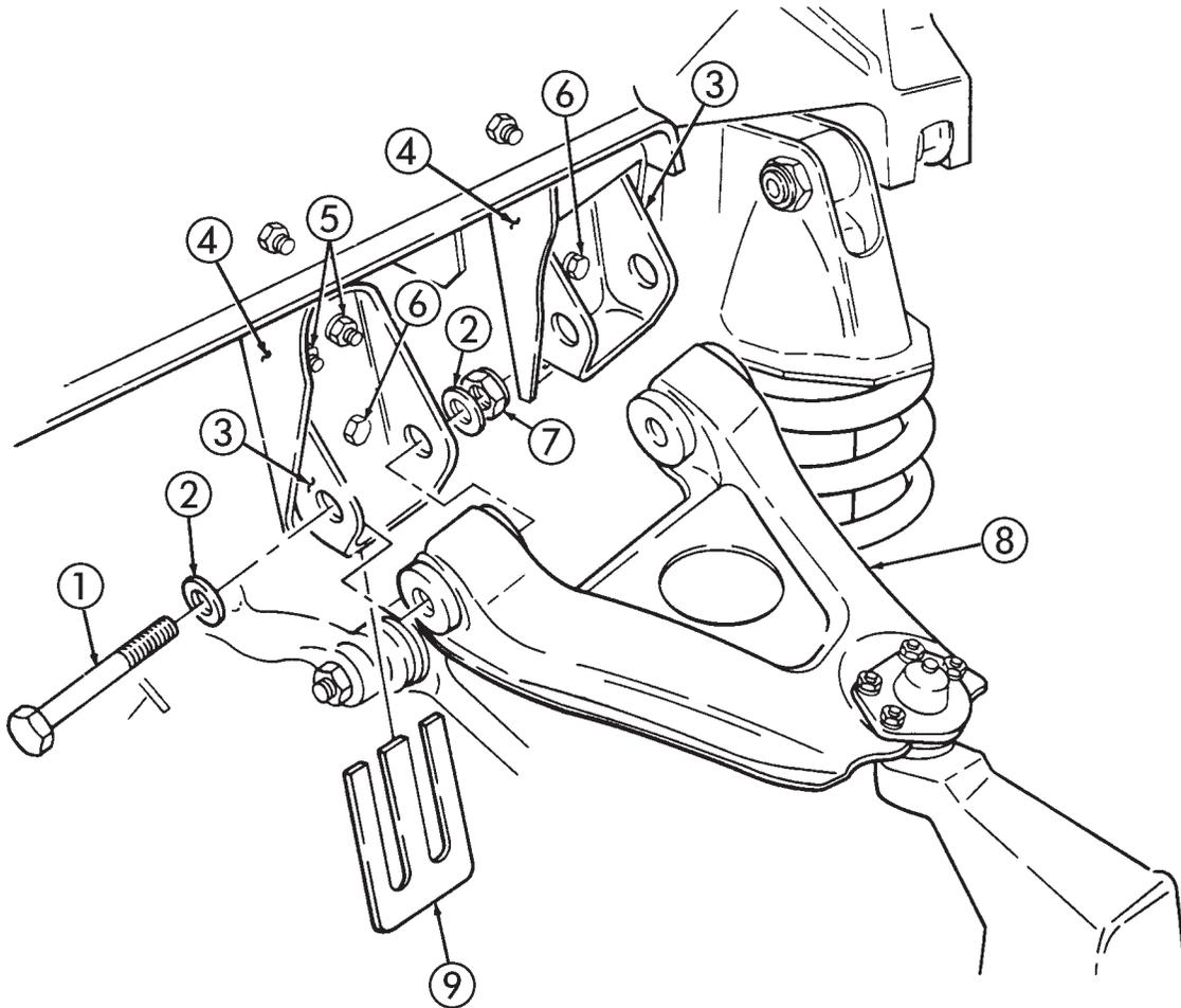
Figure 7-14 (Repeat). Caster and Camber Adjustment.
