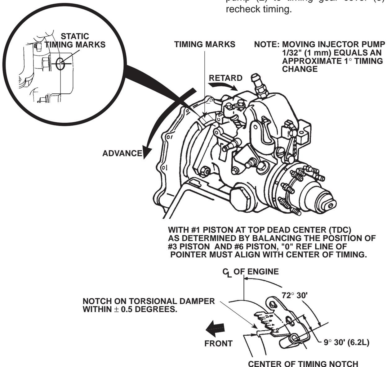
Figure 4-6. Timing Adjustment.
