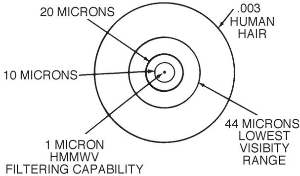
Figure 3-15. Relative Size of Micron Particles
