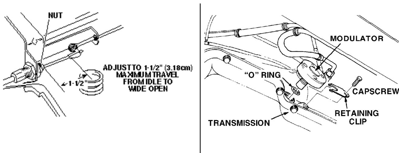
Figure 6.3. Modulator Maintenance and Adjustment.
