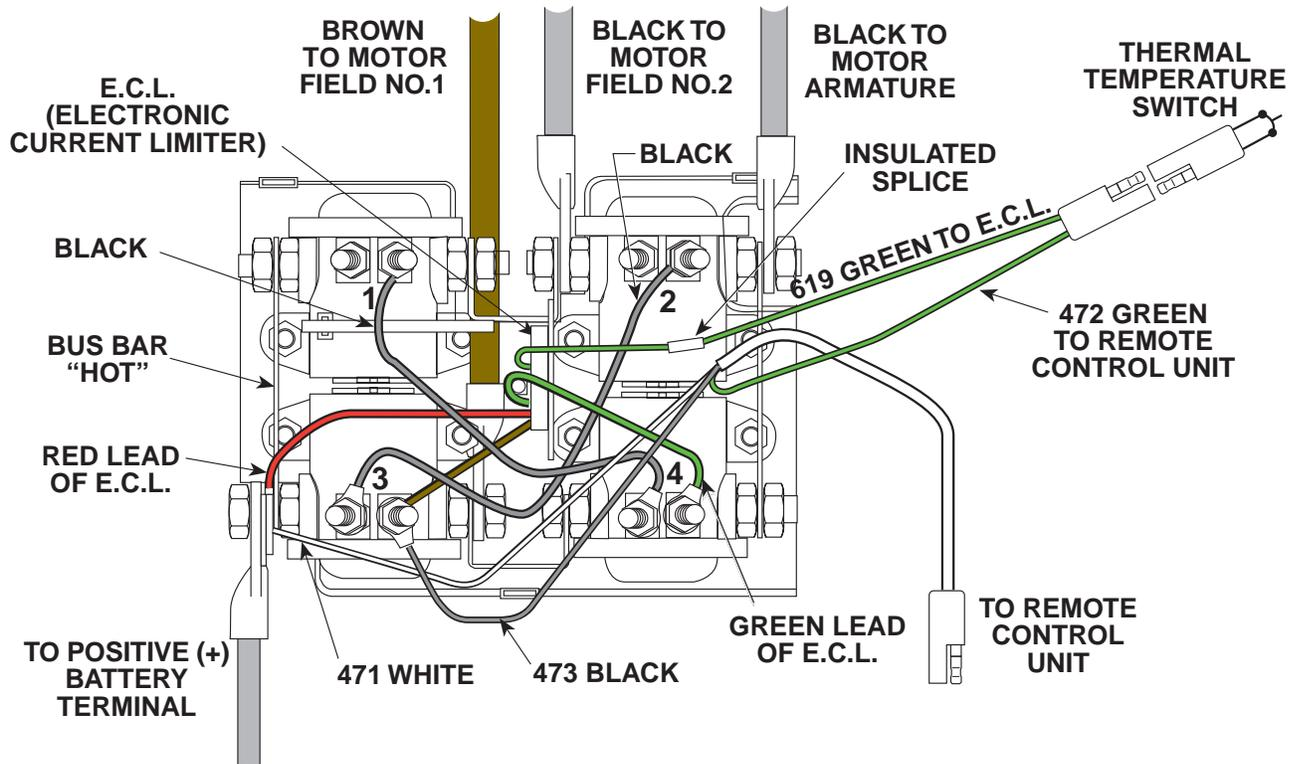
Figure 12-16. Winch Testing.
