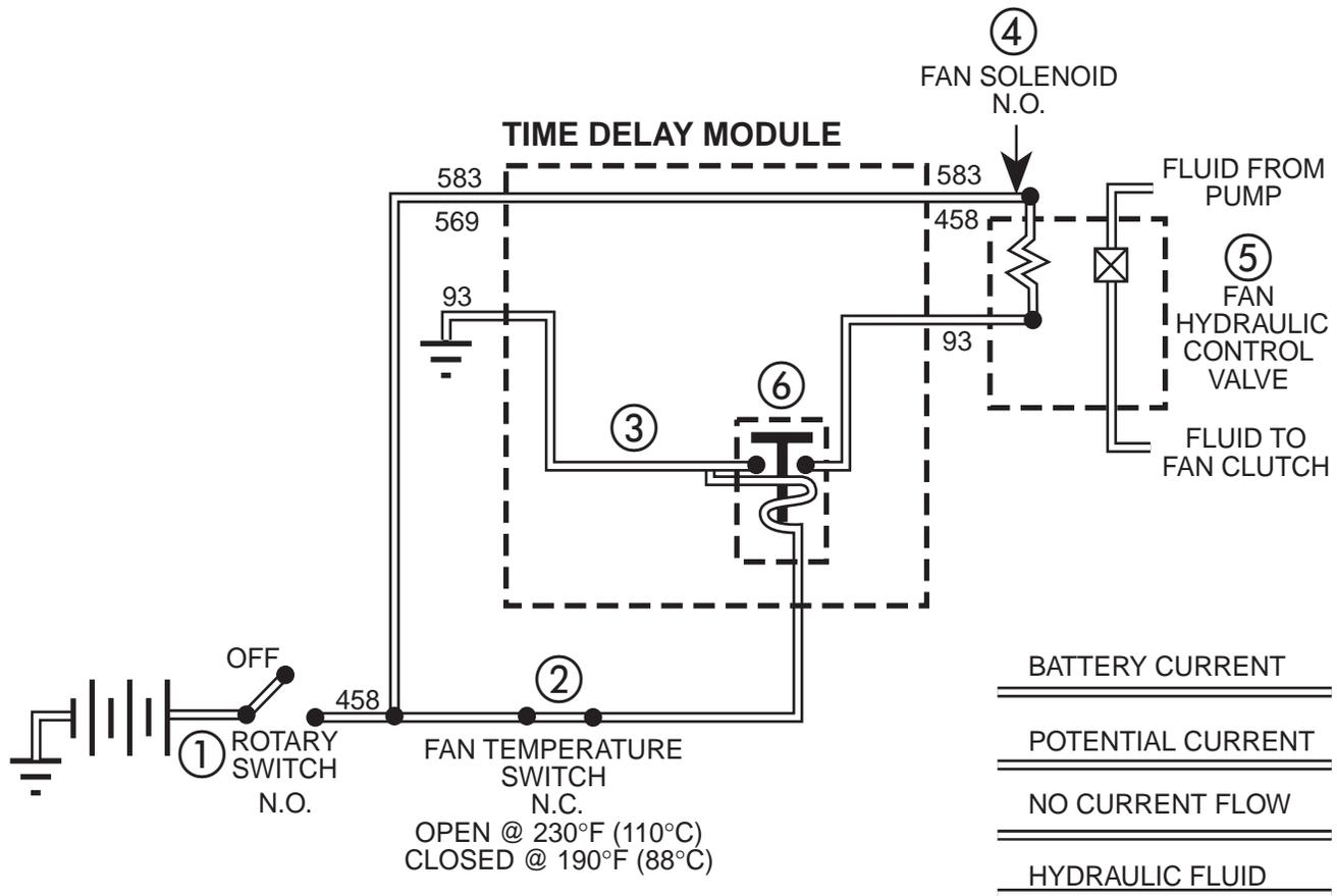
Figure 13-1. Fan Temperature Switch Closed
