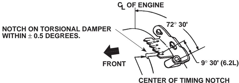
Figure 4-10. Timing Adjustment.
